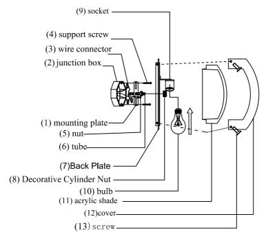
Please turn off power to the outlet and review instructions before installation. The installation must be handled by a qualified licensed electrician. Also, be sure to turn off power before changing the bulb or cleaning the fixture.
