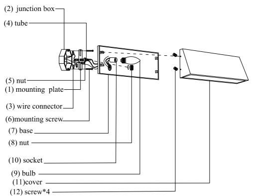
Please turn off power to the outlet and review instructions before installation. The installation must be handled by a qualified licensed electrician. Also, be sure to turn off power before changing the bulb or cleaning the fixture.
